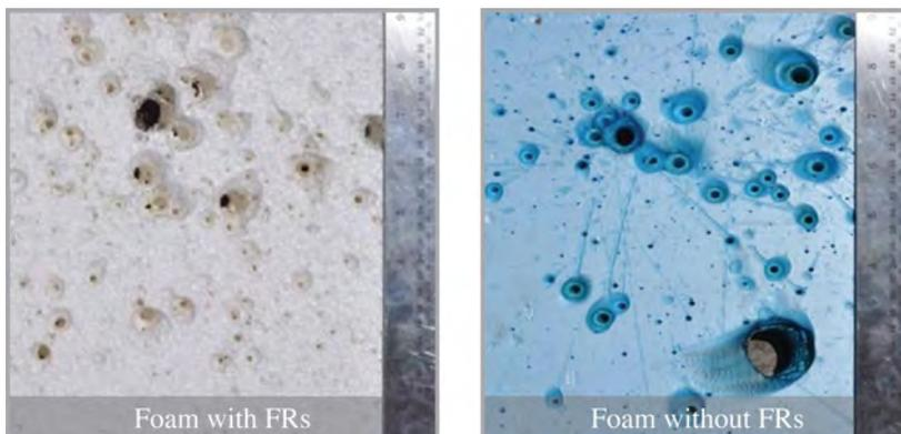
**Figure 6.** Steel welding slag dropped from approximately 4 feet onto foam with (left) and without (right) FRs. The larger hole in the sample on the right burned briefly before self-extinguishing.
