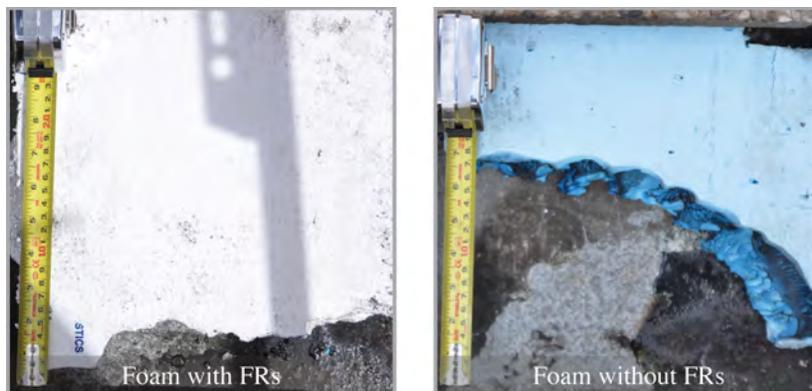
**Figure 3 (images shown to scale).** Flame propagation below the slab for small flame ignition without external heat flux. Small flame ignition of the foam with FRs (left) was not successful. Foam without FRs (right) propagated approximately 7" from the slab edge before self-extinguishing. Pavers were removed after test to show extent of burning.
