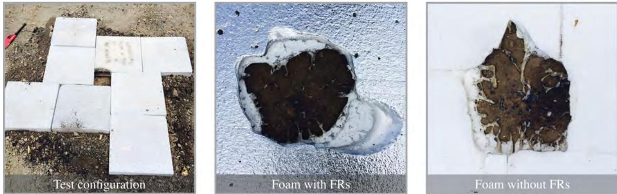
**Figure 2.** Concrete pavers cover foam plastic with a 4" x 4" opening where small butane torch was applied (left). Center image shows foam with FRs after the test; image on the right shows comparable melting of foam without FRs after the test.
