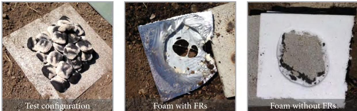
**Figure 1.** Concrete paver supports a charcoal fire above a sample of foam plastic insulation. After termination of the test, foam without FRs (left) and foam with FRs (right) displayed similar melting.
