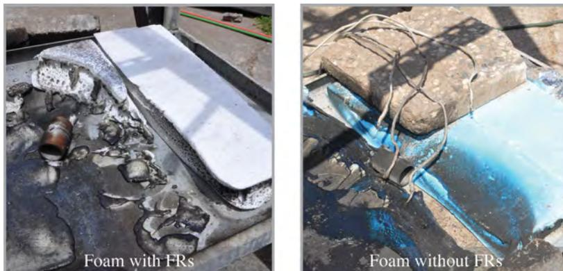
**Figure 4.** Flame spread testing with an external radiant flux above 2" concrete pavers resulted in similar flame spread rates for foam with FRs (left) and foam without FRs (right).
