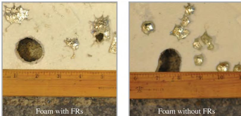
**Figure 5.** Brazing solder drips onto foam with FRs (left) and foam without FRs (right). Neither showed ignition.
